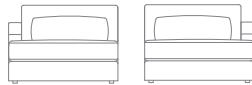
LEFT OR RIGHT ARM CHAISE AND HALF 51" w x 72" d x 36" h seat width: 45"; seat depth: 50" seat height: 19"; arm height: 24" COM 14.5 yds
